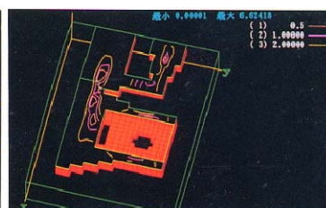
Fig. 4 修正温度勾配 G/\sqrt{R} ( \sqrt{^{\circ}\text{C}\sqrt{\text{min}/\text{cm}} ) 引け巣発生予想位置 G/\sqrt{R} \leq 1.0 (Shrinkage portion G/\sqrt{R} \leq 1.0 )
